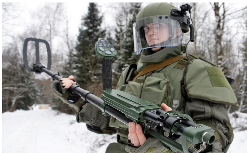
Picture 2 – Selective portable induction mine detector IMP-S2
